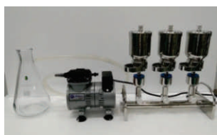
Manifold with vacume pump
